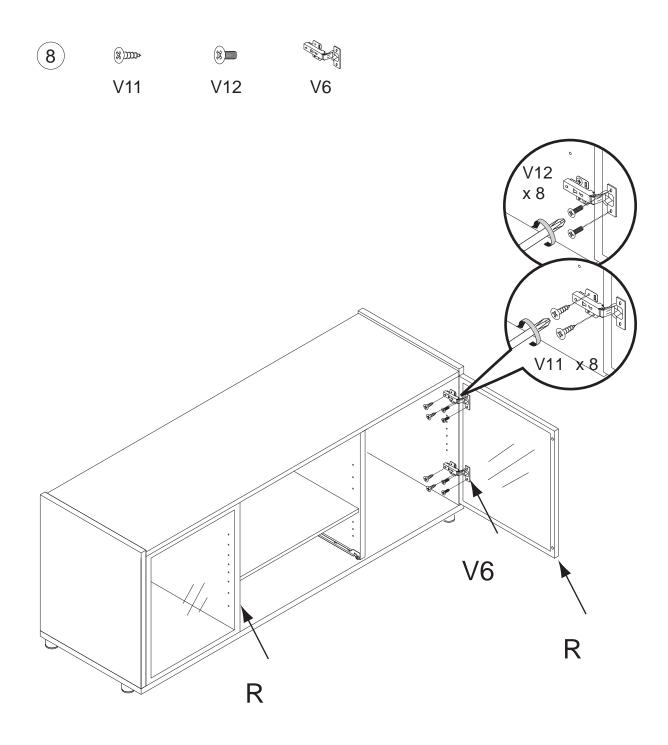
8. Place the hinge(V6) onto the aluminum frame of the door(R)with screws(V12) and then fix the door(R) onto the TV cabinet with screws(V11).
